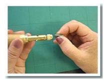
2. Install the blade in the top of the main body.
