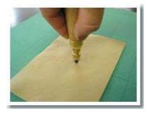
4. Release pressure when the blade penetrates the material.
