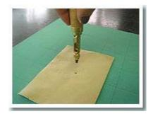
5. When you have cut the hole, pull the punch out of the material. The cut out circle of the material will remain in the blade, but if you continue to cut, the remains will begin coming out from the side of the tool.
