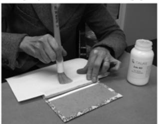
TIP: Make sure to completely cover Supercloth as this will act as the chief means of support between the block & case.
