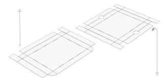
Pre-crease all lines prior to snapping any walls into place. Pay extra attention to the double crease lines which are approximately 1/4" apart along doubled over the walls. It is critical that both crease lines are folded at a full 90° or more.
