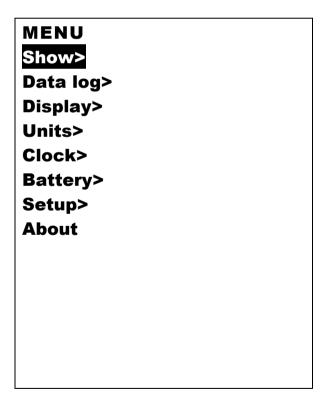
The first menu item "Show" is highlighted, different menu items can be highlighted using the  $\uparrow$  and  $\checkmark$  buttons. The wanted action is done by highlighting the appropriate menu item and pressing the Set button. To abort without doing anything press the X button. In some cases a further sub-menu is displayed with more choices.
