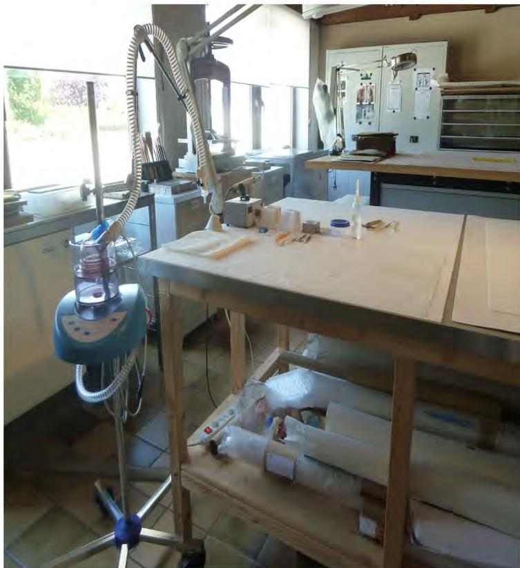
Put the tube into the clasps while preparing your object and every time when you are not holding it in your hand to work – and always bend the flexible end of the arm in a way, that it points downwards and away from your object.
