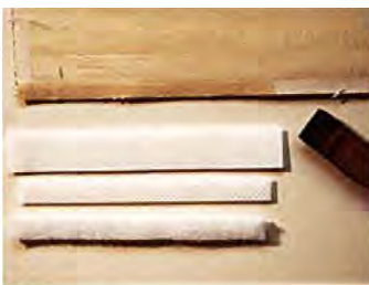
Moistening process of the poultice material. Top: Paper interleaf Middle: Enzyme poultice
