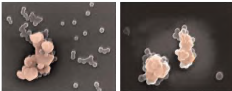
Figure 1: Left picture shows a SEM micrograph (50K magnification) of TiO 2 dispersed in a conventional acrylic latex polymer. Picture on right shows TiO 2 dispersed in AVANSE™ MV-100 Resin. The latex particles appear as the smaller, gray spheres, and TiO 2 appears as pink.
